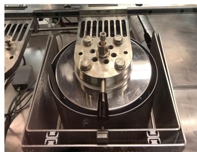
Fig. 2 Custom made High Temperature Electrochemical Cell (HTEC) for electroreduction.
