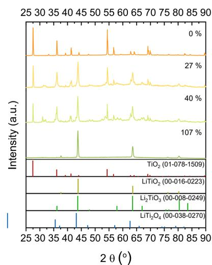
Fig. 4 XRD patterns of the oxide feeds after electrolysis (corresponding to the following percentage of the theoretical charge 0%, 27%, 40%, and 107%.)
