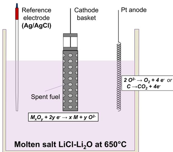
Fig. 1 Schematic representation of the electroreduction process.
