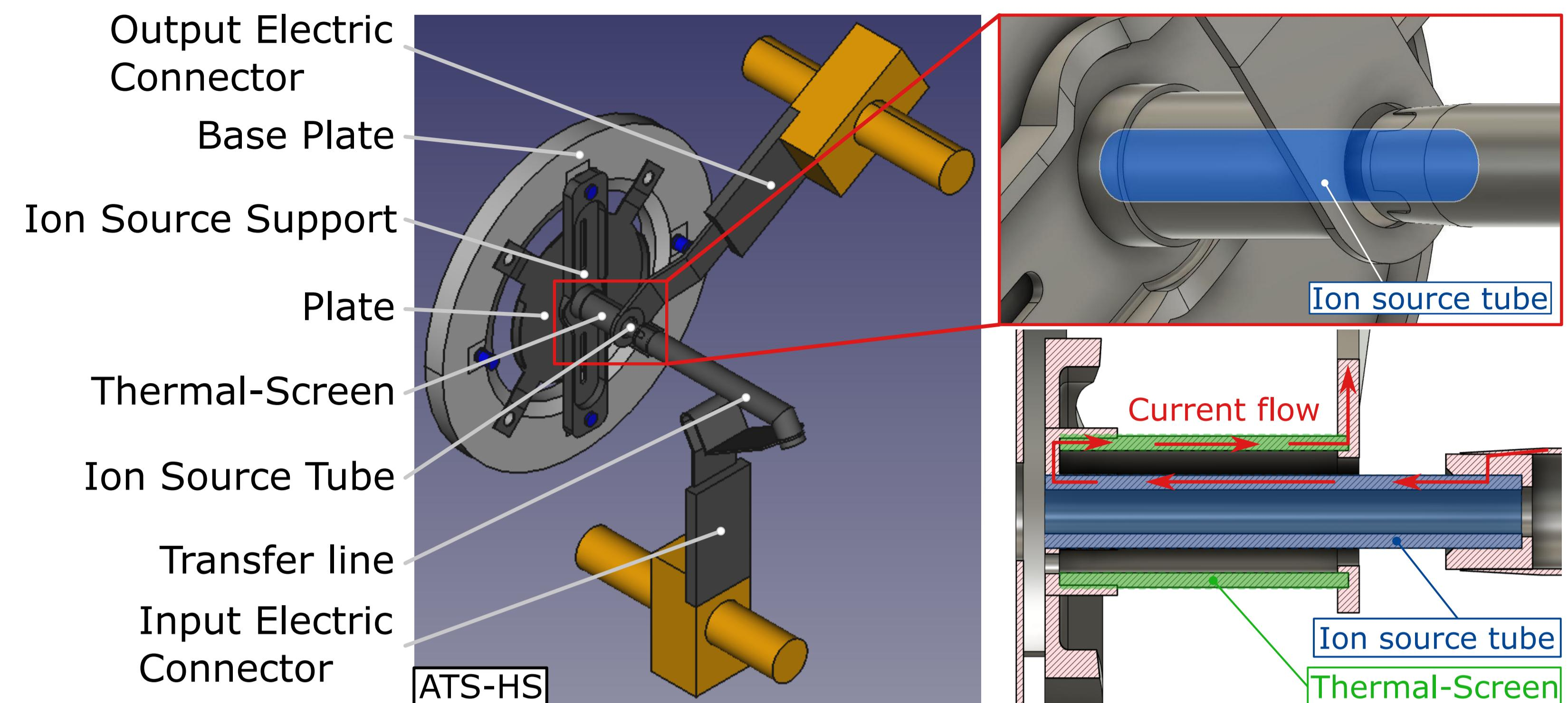
⚡ Add a second feedthrough for the heating system electrical current : one input & one output.
