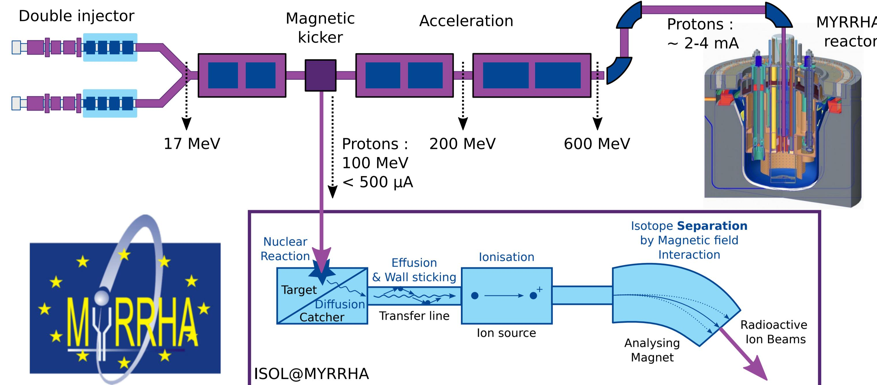
**ISOL@MYRRHA:** will extract part of the proton beam coming from the accelerator and use it to produce Radioactive Ion Beams (RIBs) with the Isotope Separation On-Line (ISOL) technique.
