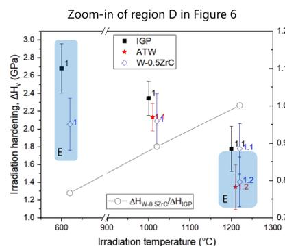
Fig 10. Comparison of irradiation hardening vs. temperature for the samples irradiated up to 1-1.2 dpa.
