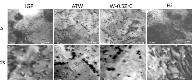
Fig. 5 The TEM images of dislocation loops (DLs) and voids induced by ion irradiation [4]
