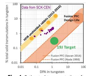
Fig. 4. Estimated transmutations for tungsten irradiated in different reactors [3]
