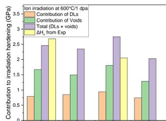
Fig. 6. The contributions of defects on irradiation hardening
