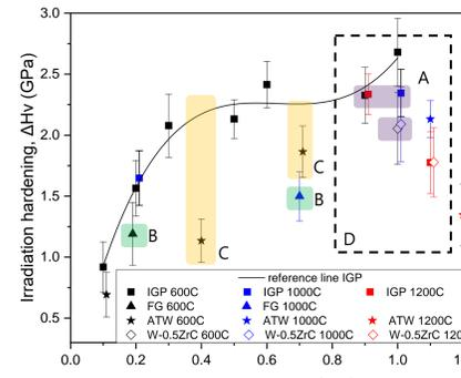
Fig 9. The irradiation hardening vs. irradiation dose.
