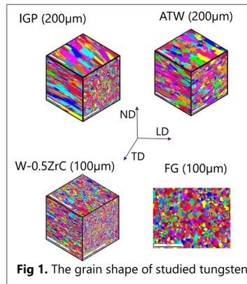
Fig 1. The grain shape of studied tungsten
