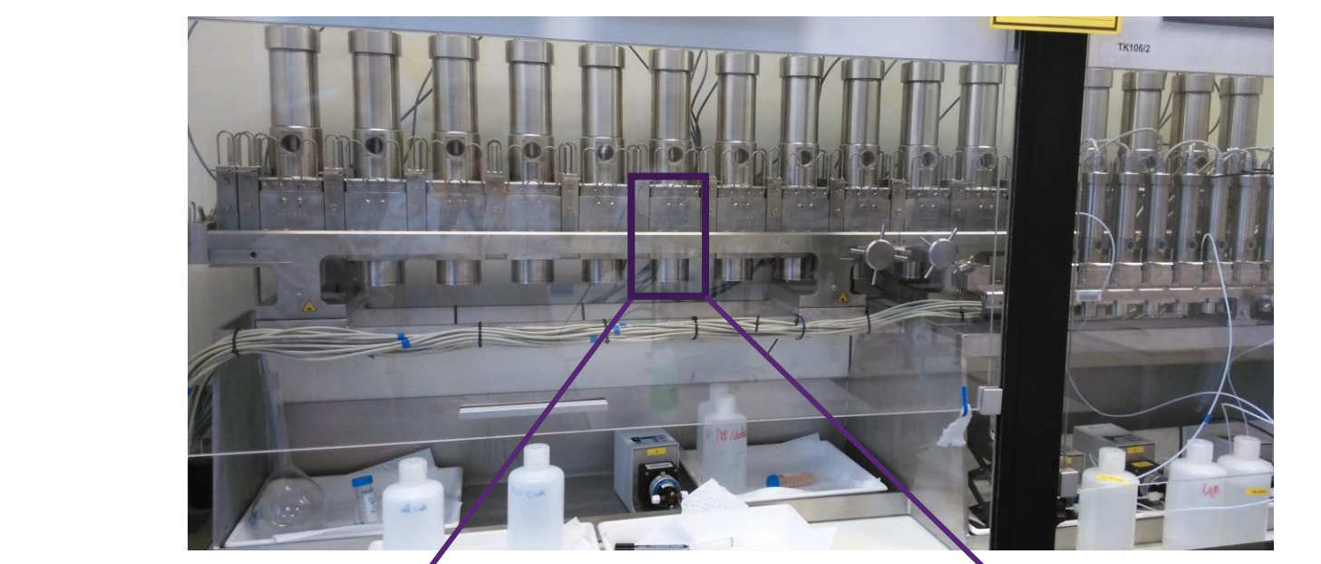
Figure 2: 16 stage annular centrifugal contactor setup
