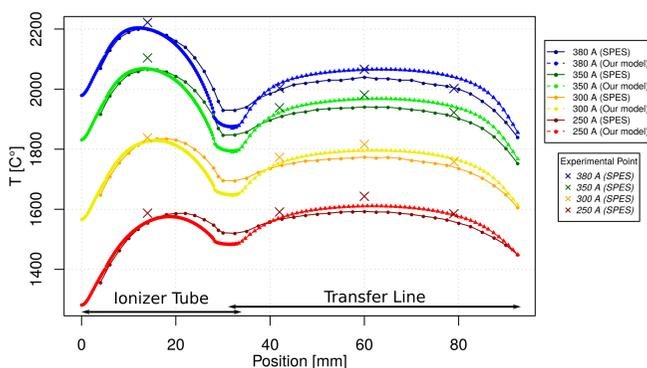
Figure 1: Temperature comparison between SPES and our model of ANSYS simulation results along the ionizer tube [0-33 mm] & the transfer line [30-95 mm]
