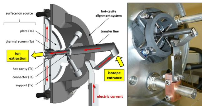
The electrical clamp is copper, the rest of the heating system is **tantalum** which has good properties for surface ion source: High work function ( $\phi=4.19$  eV), High melting point ( $\sim 3000^{\circ}C$ ).
